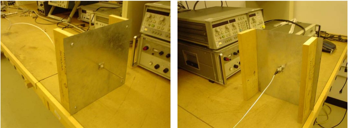
Fig. 2.7 Monopole antenna on a small square ground plane.
