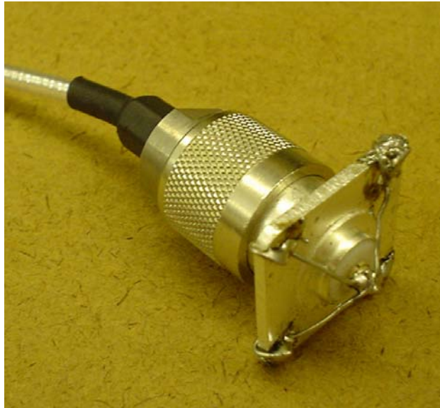
Fig. 2.8 Bulkhead connector with a short-circuit to ground.
